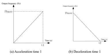
Fig. 7-9 Acceleration and Deceleration Time
