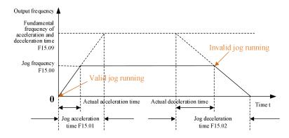
Fig. 7-32 Schematic Diagram of Jog Running
