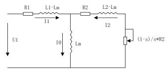
Fig. 8-18 Equivalent Circuit of Three-phase Asynchronous Motor
