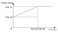
Fig. 7-17 Schematic Diagram of Analog Output of Count and Length
