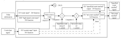
Fig. 7-42 Block Diagram of Counting Function
