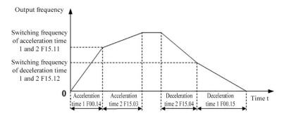
Fig. 7-34 Schematic Diagram of Automatic Switching of Acceleration and Deceleration Time During acceleration, if the output frequency is less than the switching frequency of the acceleration time 1 and 2 (F15.11), the acceleration time 1 will be the current valid acceleration
