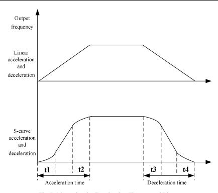
Fig. 7-16 Acceleration/Deceleration Time Control Diagram
