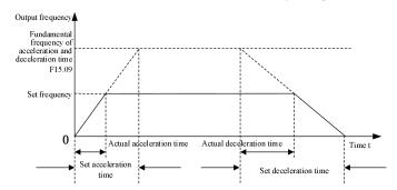
Fig. 7-33 Schematic Diagram of Acceleration and Deceleration Time
