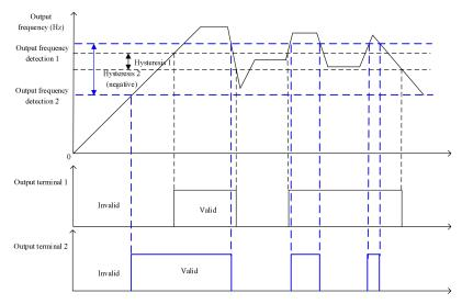
Fig. 7-37 Schematic Diagram of FDT Detection
