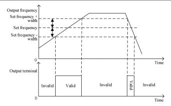
Fig. 7-36 Schematic Diagram of FAR Detection
