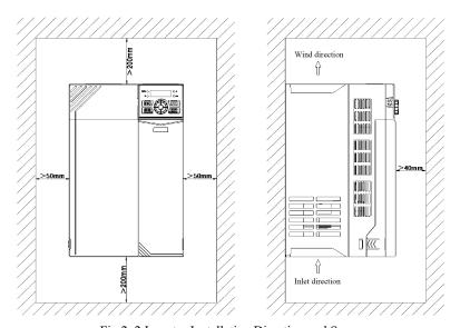
Fig.2-2 Inverter Installation Direction and Space
