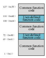
Fig. 12-21 Classification of MODBUS Function Codes
