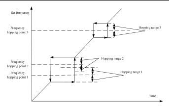
Fig. 7-35 Schematic Diagram of Frequency Hopping
