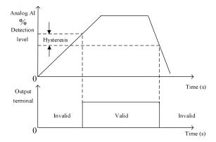
Fig. 7-38 Schematic Diagram of ADT Detection
