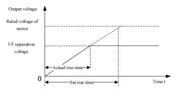
Fig. 7-20 Rise Time Description of VF Separation Voltage
